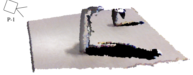
Figure 3: The point cloud as seen by the robot in Figure 1 and in the first perspective in Figure 2. The dark edge is the long edge of the table faced by the robot. Black color indicates shadow areas. Note that the sugar pack and mug handle are not visible.
