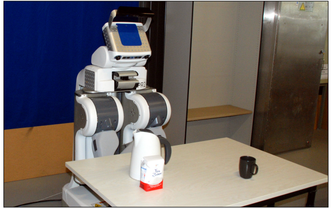
Figure 1: A PR2 robot looking at a table. From the current perspective, the sugar pack is occluded by the coffee pot and the handle of the mug is not visible, causing the robot to confuse it with a cup. From a different perspective, however, the robot would see the sugar pack and recognize the mug correctly. That is, sensings from different perspectives are inconsistent.
